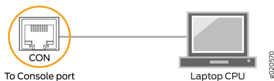
Figure 53: Connecting a Device Directly to a Management Console
