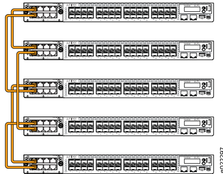
Figure 42: EX4550 Switches Mounted on a Single Rack and Connected in a Ring Topology Using 8-port 10GBASE-T Expansion Module and Using Short and Medium Cables
