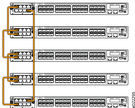
Figure 41: EX4550 Switches Mounted on a Single Rack and Connected in a Ring Topology Using 8-port 10GBASE-T Expansion Module and Using Short and Long Cables: Example 2
