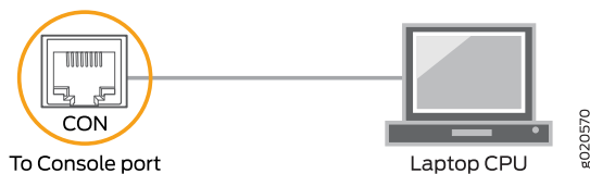
Figure 41: Connecting a Device Directly to a Management Console
